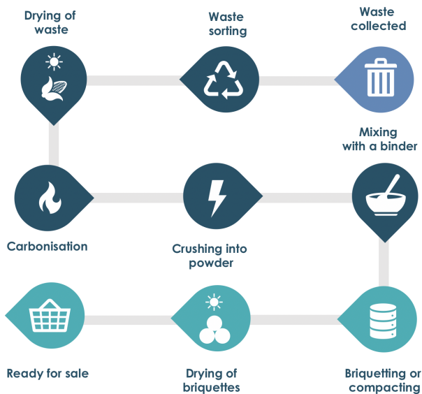
Figure 1: Diagram of the briquette-making process (Image by Urban Action Lab/KNOW, 2020)
